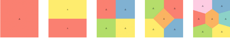
Fig. 7. Plot of the Lloyd's centroidal power diagrams for n = 1, 2, 4, 5, 7 cells from left to right.
